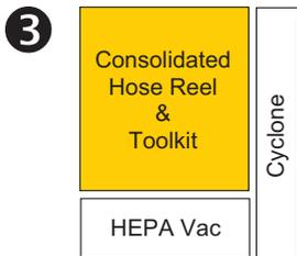
In this configuration the Consolidated Hose Reel & Toolkit (CTK) rides atop the vacuum creating a single unit for easy deployment and storage.
