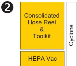
The Consolidated Hose Reel & Toolkit (CTK) provides storage for vacuum hoses, compressed air lines, sanders, tools, and abrasives. It's available with or without casters, and can ride atop the vacuum.
